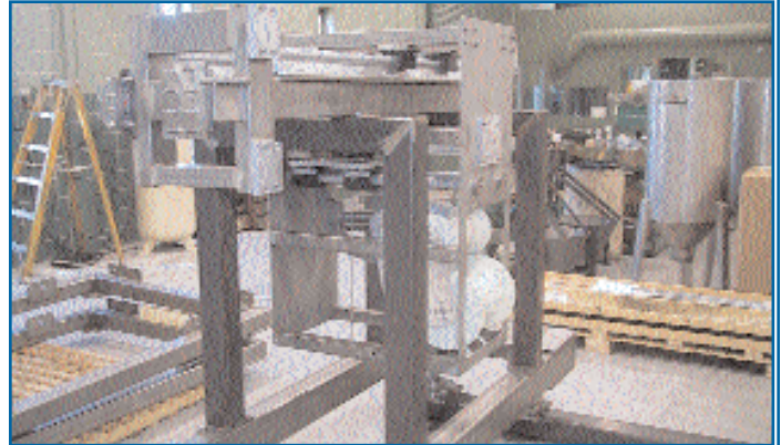
Gear head and blade housings being built for JCK-1 number 3.
